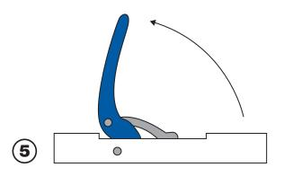
To remove excess water, pull back the lever until the rollers move over the sponge, squeezing out all the water, then return to the hold position. (But not back to Step 1 as this allows the sponge to be released).
